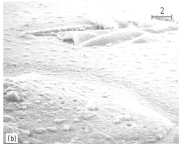
Figure 13 (a) Tears in the silane layer in specimen TF-50 °C, (b) Tears in the silane layer and in the interphase in specimen TF-AC, (c) Higher magnification of the left-hand corner of the torn region in (b). (Scale bar in μm.)
